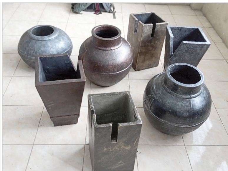
Figure 3: Results of GFRC training in the form of pots Source: A photo by Handoko (2021)
