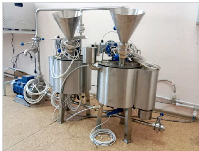
Figure 2: Hydrodynamic Extraction Setup Source: Authors' own research
